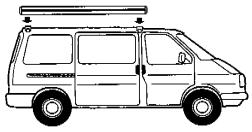
C. Set the brackets so that the underside of the bracket is placed 10mm above the roof edge. NOTE: THE FRONT BRACKET MUST BE POSITIONED ON THE DOOR POST BETWEEN THE SLIDING DOOR AND THE FRONT PASSENGER DOOR. MAKE SURE THAT IT DOES NOT INTERFERE WITH DOOR OPERATION! POSITION BACK BRACKET JUST BEHIND THE REAR SIDE WINDOW.
