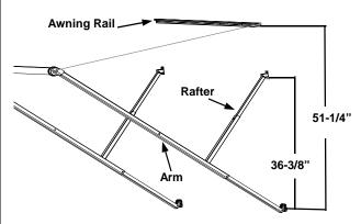
**C.** Position the bottom bracket of the arms so that the previously made marks line up with the center line of the bottom bracket bolt.
