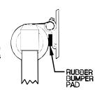
**D.** Align arms vertically and install the bottom brackets using the #12 x 1" screws provided.
